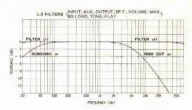
To remove such harmful ultra low frequency noises with the least effect on the audible frequency range, this unit is provided with the Subsonic Filter.
